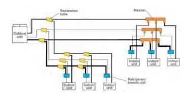
Figure 6: Typical Layout of a VRF System (taken from ASHRAE)
